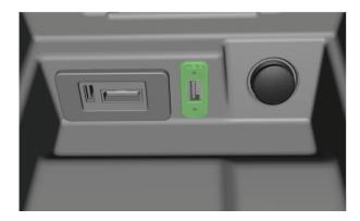
5. Go back to the IDCORE home screen on the interface menu, plug your phone into the USB socket in the via a suitable USB cable.
